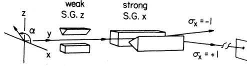
Figure 6.4 The modified SG apparatus to observe and measure the weak value for spin-1/2 particles. The diagram clearly shows the three stages of the weak measurement process; preparation, weak and strong (Duck *et al* 1989).
