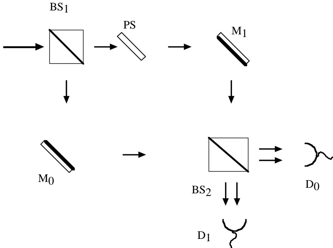
**Fig. 1** A Mach-Zehnder interferometer splits the single-photon wavepacket into two packets traveling two paths at the first beam splitter, BS<sub>1</sub>. The phase of one wavepacket may be shifted at PS. Those two wavepackets will be overlapped if the second beam splitter, BS<sub>2</sub>, is present, before reaching one of the detectors.
